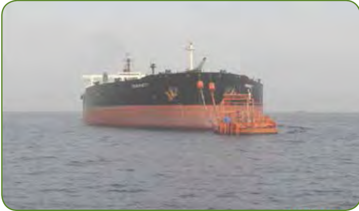
Crude Oil unloaded from VLCC on high seas at SPM of MRPL located 16 km from the shore of New Mangalore Port.
